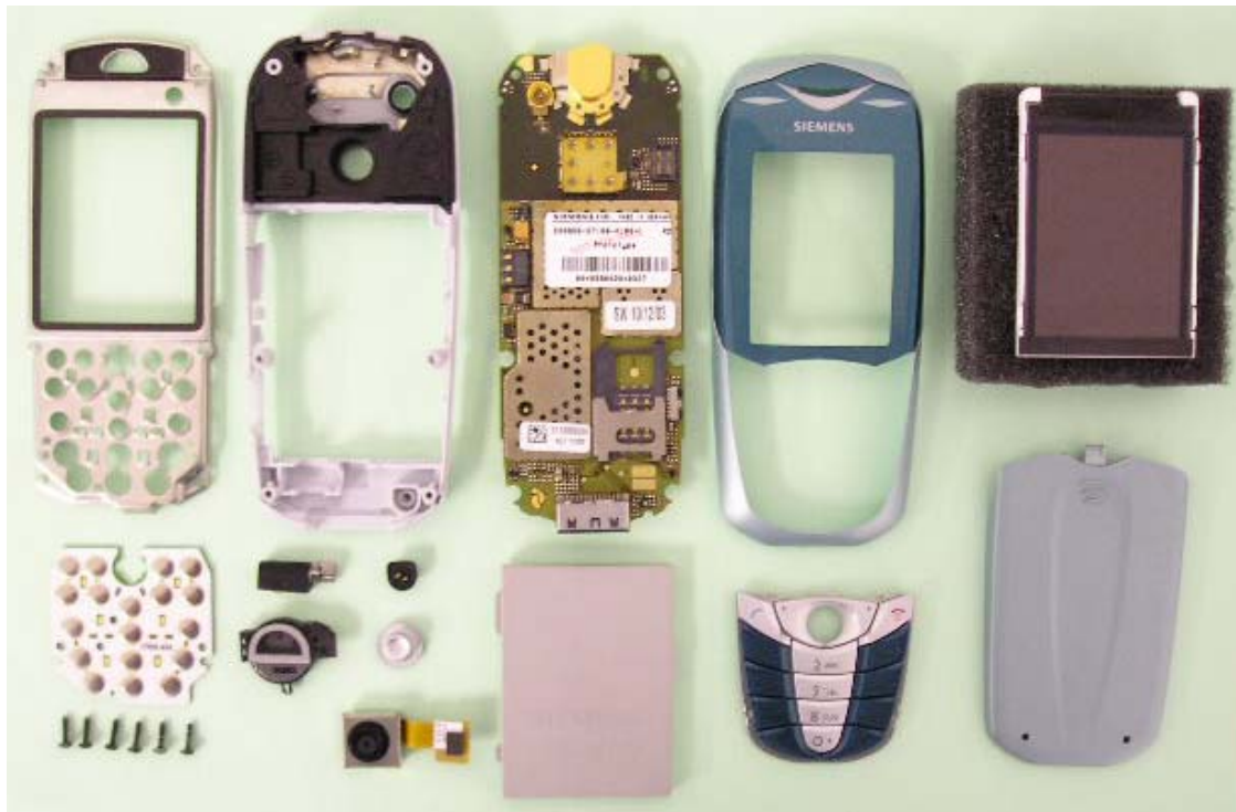
Fully disassembled CX65
